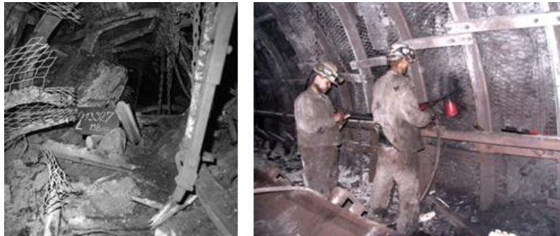
Fig. 3 Rockburst consequences (left) and continuous rockburst prognosis – drilling tests (right)
